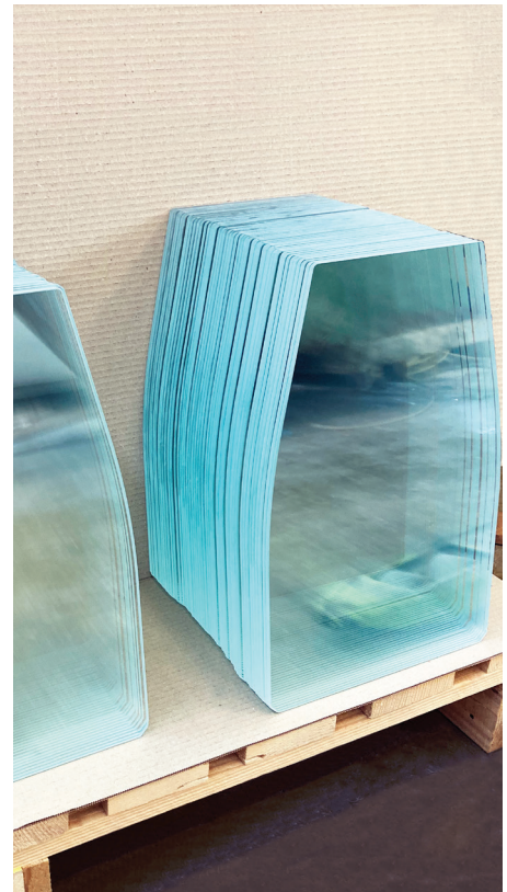
Each glass is individually CNC drilled and the edge is ground, which increases the lamp's durability.
