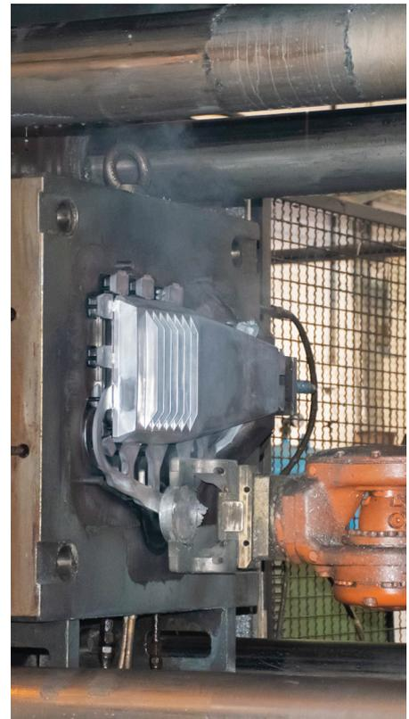
*Bühler 840 SCD die-casting machine has more than 950 tons of closing force with an automatic robotic ejector arm.*
