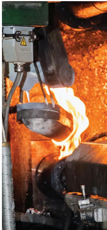
*Aluminum alloy is heated to more than 700 degrees Celsius and is transported with automated robotic arm.*
