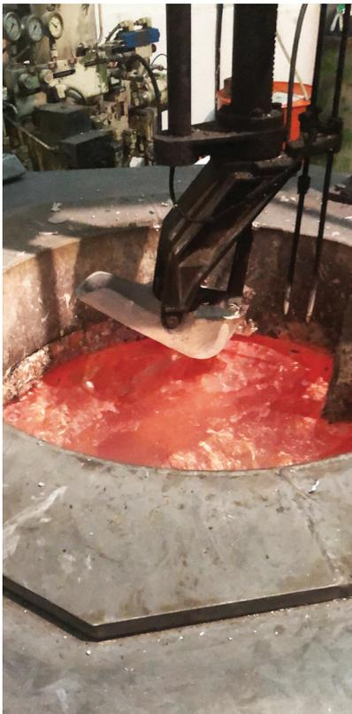
*Material used for die casting is EN AC 47100 (DIN 231 D) - AlSi12Cu1(Fe). Used for pressure die casting with excellent machinability and hardness.*
